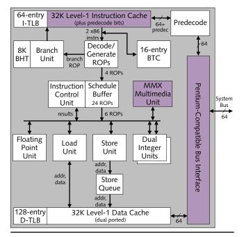
**Figure 1.** AMD's K6 can decode two instructions per clock cycle, generate four ROPs, and dispatch up to six ROPs from the schedule buffer. Purple blocks are changed from the NexGen 686.
