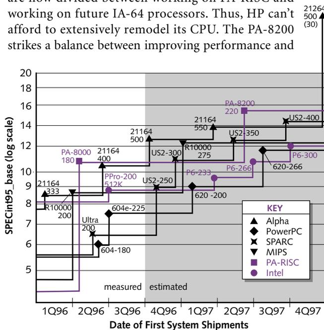
**Figure 1.** Although Digital has wrested the performance lead from HP's PA-8000, the forthcoming PA-8200 should regain the lead until Digital's 21264 debuts. (Source: SPEC, MDR estimates)
