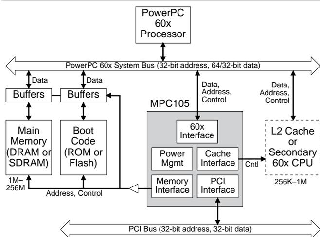
Figure 1. A typical PowerPC system using Motorola's MPC105 requires little glue logic for cache, memory, and PCI interfaces.
