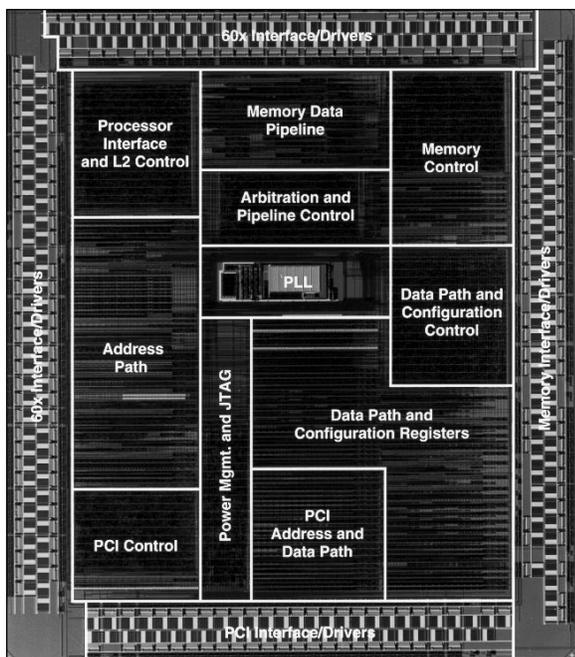
Figure 2. Die photo of the MPC105, which measures  $6.7 \times 5.8$  mm and uses about 300,000 transistors in 0.65-micron CMOS.
