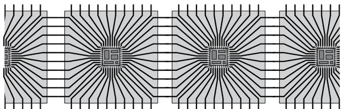
Figure 2. Top view of a set of lead frames with dice wire-bonded in place. These frames are ready to be covered with plastic to form the outer shell of the QFP part.
