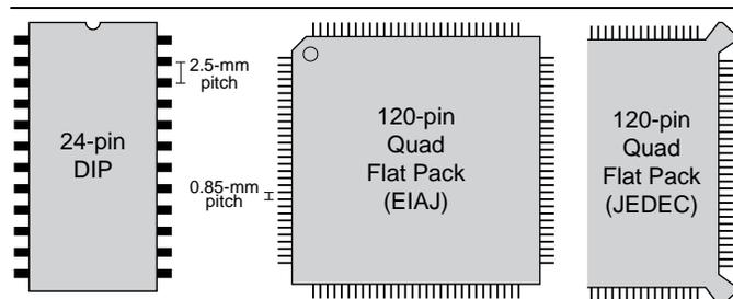
Figure 1. A quad flat pack can have many more pins than a DIP due to its smaller pin spacing. The JEDEC package differs from the EIAJ standard due to its corners. (Parts are approximately actual size.)
