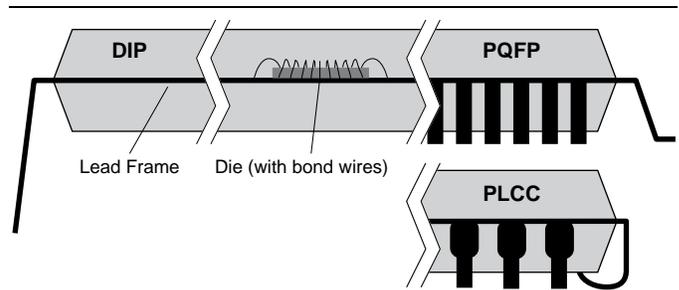
Figure 3. Side view of various plastic packages. Through-hole packages (left) use straight leads, while surface-mount packages (right) have flat leads that either spread out (PQFP) or tuck under the package (PLCC). The center section shows the die bonded to the lead frame and is common among all of these packages.
