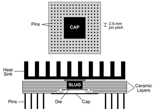
Figure 4. As shown at top, a pin-grid array (PGA) package has several rows of pins on the bottom. The cutaway view (below) shows the die mounted on layers of ceramic.
