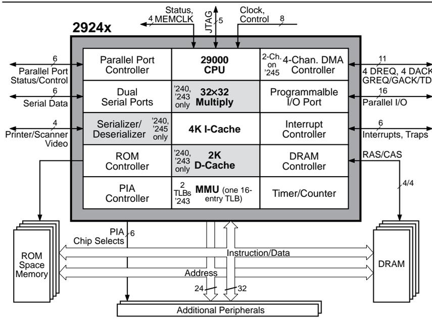
Figure 1. Block diagram of a 2924x system. The processor provides glueless interfaces to most memories and peripherals likely to be found in an embedded system.
