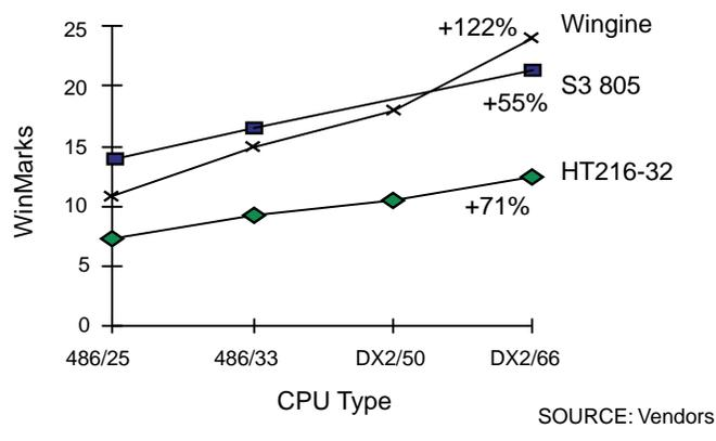
Figure 1. Graphics performance scaling versus CPU type.
