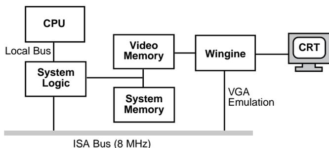
Figure 3. "Wingine" graphics system configuration.
