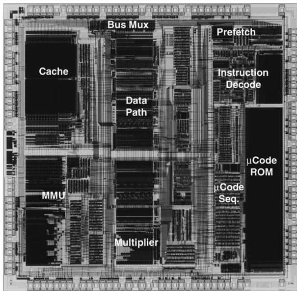
Die photo of Cyrix's 486SLC, which includes 600,000 transistors on a 410 x 410 mil (10.4 x 10.4 mm) die.
