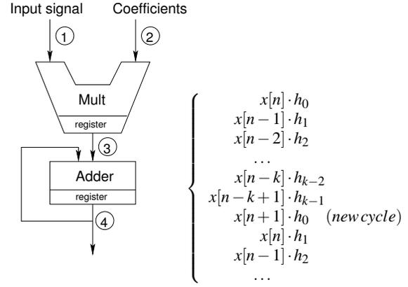
Figure 2: MAC architecture (left) and data sequence at the output of the multiplier (right).
