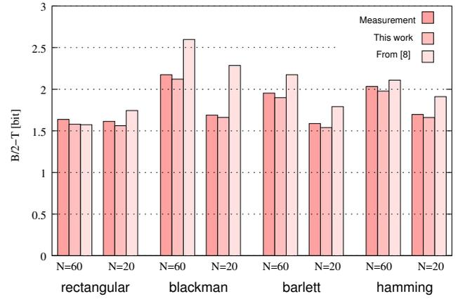
**Figure 5: Difference in the transition activity with respect to random noise for a set of low pass FIR filters designed with different windows.**
