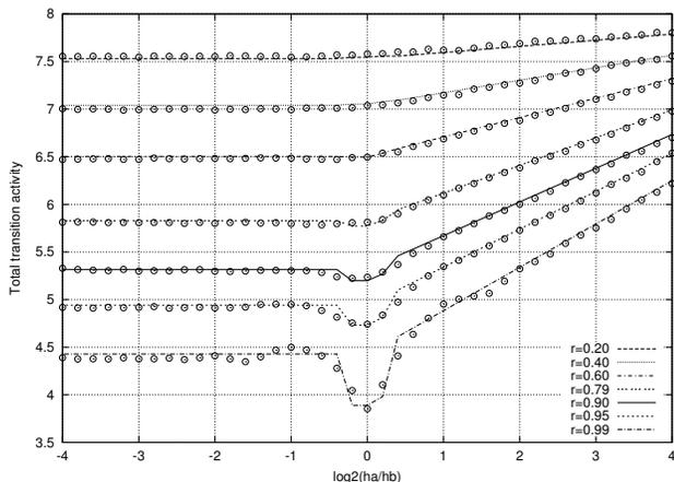
**Figure 4: Measured (dots) and estimated (lines) activity versus filter coefficients ratio for signals with different correlation factor.**
