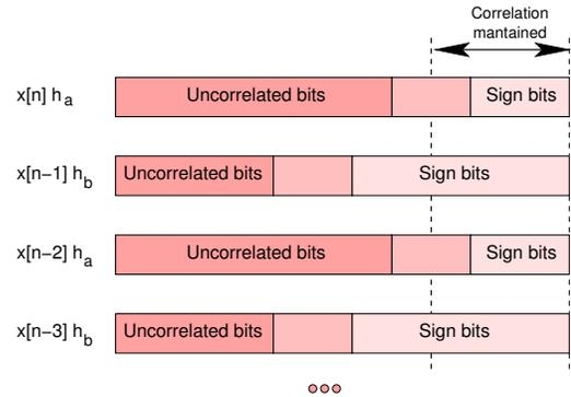
Figure 3: Correlation regions after multiplying a Gaussian signal by  $\{h_a, h_b\}$ .
