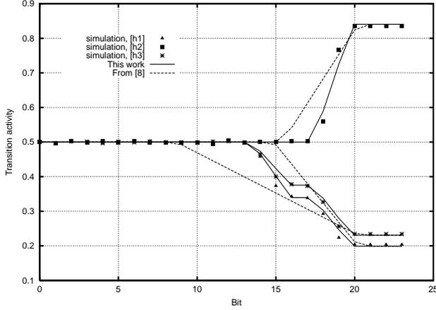
Figure 1: Comparison of the bit level transition activity estimated by [8] and this work.
