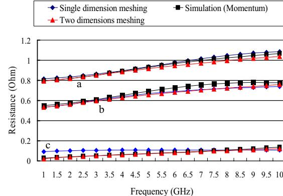
Fig. 5 Resistance of a single conductor with different width and thickness, (a)  $w=10, t=1$ , (b)  $w=15, t=1$ , (c)  $w=100, t=13$ . (unit:um)
