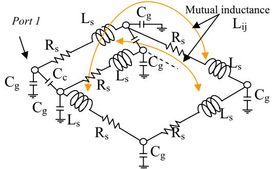
Fig. 2 Equivalent lumped circuits for inductor.
