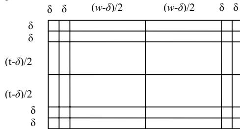
Fig. 3 A conductor with non-uniform meshing.
