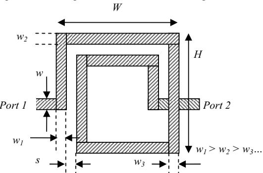
Fig. 1 Inductor layout (top view) and related parameters.
