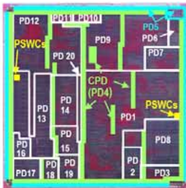
Fig. 3. Mobile processor with module-level Run-Time Power Gating.
