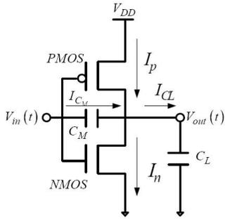
Fig. 1. CMOS inverter model.
