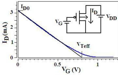
Fig. 7. The approximation of PMOS transistor drain current.
