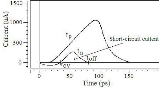
Fig. 4. Output current evolution in NMOS and PMOS transistors for a falling input voltage.
