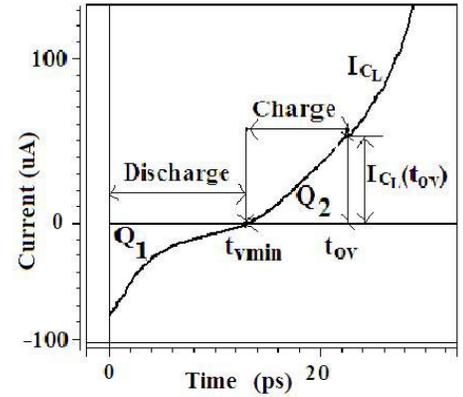
Fig. 6. The approximation of the current  $C_L$  during  $t_{ov}$ .
