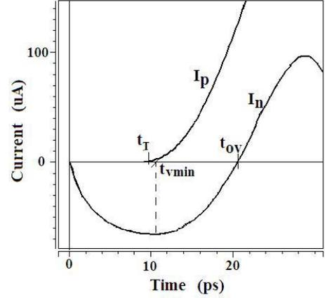
Fig. 5. The PMOS and NMOS transistor drain currents  $I_p$  and  $I_n$  during  $t_{ov}$ .
