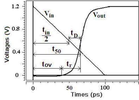
Fig. 2. The output voltage of CMOS inverter for a falling input.
