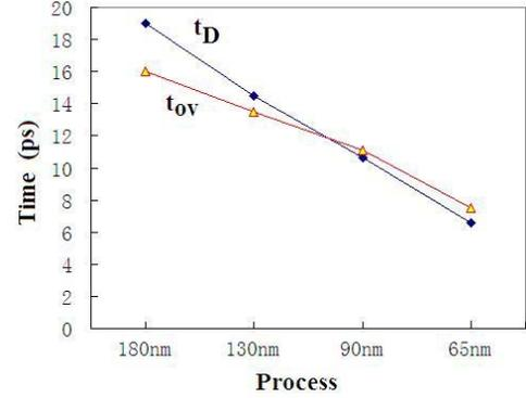
Fig. 3. Gate delay  $t_D$  and overshooting time  $t_{ov}$  with various process.
