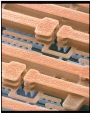
**Figure 1:** Sub-nanometer image of copper interconnect
