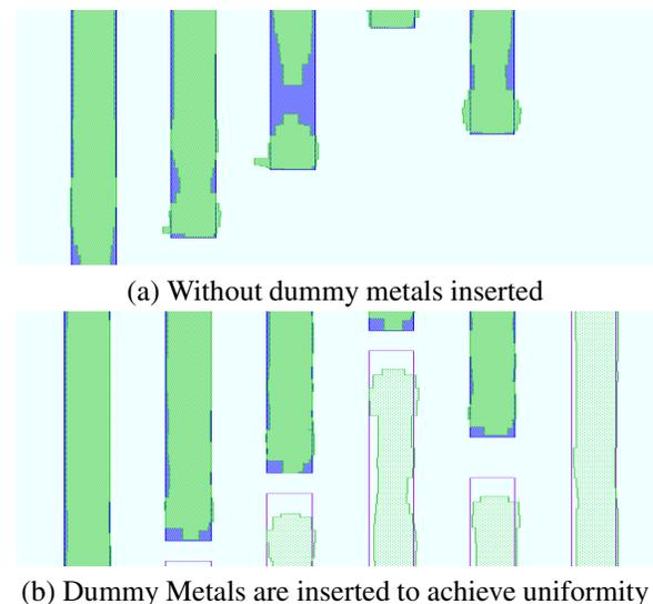
Fig. 1. Simulation results from Calibre. Without dummy metals inserted, the wires cannot be printed correctly even after OPC in (a). With dummy metals inserted, there are very little errors in (b). Defocus is considered in the aerial image simulation.
