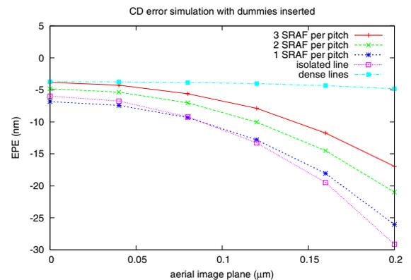
Fig. 2. Simulation results of DOF. The dense lines have the smallest EPE across all defocus levels and hence the best DOF. A larger EPE indicates a larger critical dimension (CD) error.
