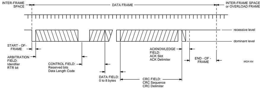
Figure 1. CAN Data Frame (Source [9]) .
