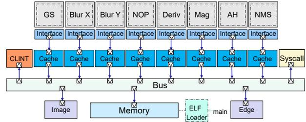
Fig. 3. Modeled shared memory processor. The blue lines represent SystemC blocking transport calls ( $b\_transport$ ).
