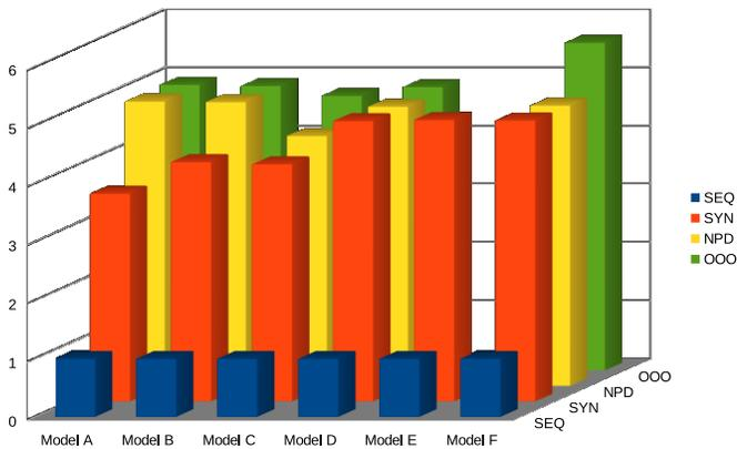
Fig. 6: Simulation speedup for different parallel simulation modes on a 16-core host
