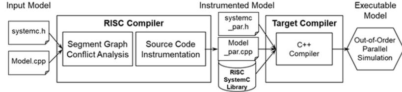
Figure 2: RISC Compiler and Simulator Flow [14]
