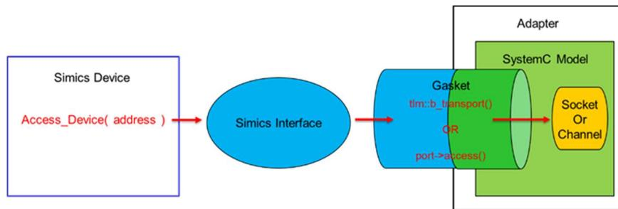
Figure 6: Simics-to-SystemC communication
