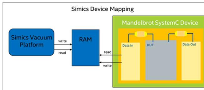
Figure 9: Simics Device set up for Mandelbrot Renderer example
