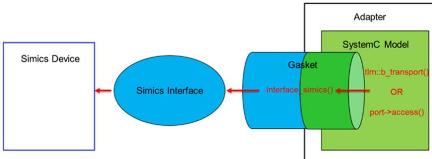
Figure 7: SystemC-to-Simics communication
