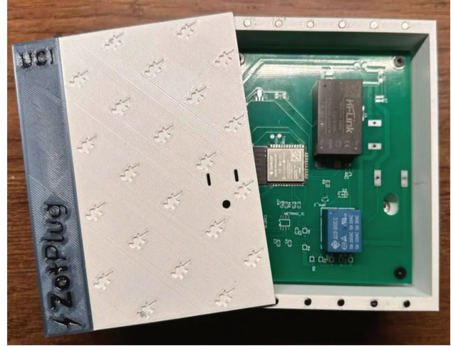
Figure 9: Early Printed Circuit Board Prototype with Integrated 3D-Printed Enclosure. This intermediate Winter Quarter prototype represents the first surface-mount implementation of the hardware design and served as an important evaluation stage prior to transitioning to the final perfboard-based implementation.
