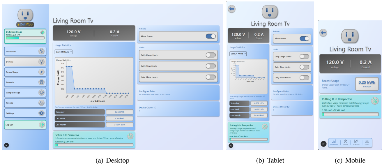
Figure 7: Winter Quarter Device Level Monitoring Interface Across Multiple Devices for Detailed Energy Analysis. This view provides users with detailed statistics for individual ZotPlug devices, including energy consumption trends, historical usage metrics, and interactive controls for device-level monitoring and analysis.
