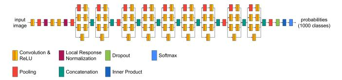
Figure 3: GoogLeNet CNN structure, redrawn from [5].
