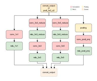
Figure 4: The structure of the inception blocks inside the GoogLeNet CNN, redrawn from [1].
