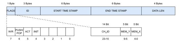
Figure 17: Memory access encoding inside the mari.log binary file.
