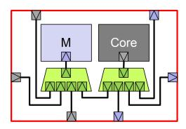
Figure 1: R-type cell inside the GPC architecture, redrawn from [7].
