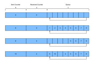
Figure 16: Example of ring buffering inside an 8-byte long FIFO.
