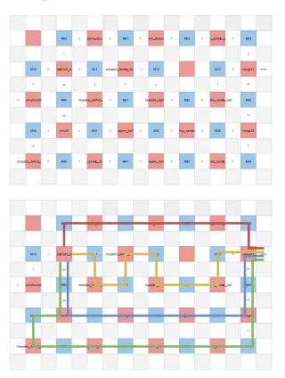
Figure 11: GoogLeNet CNN on GPC (version 1) spreadsheet description of the first inception block. The four paths are highlighted in the bottom image.
