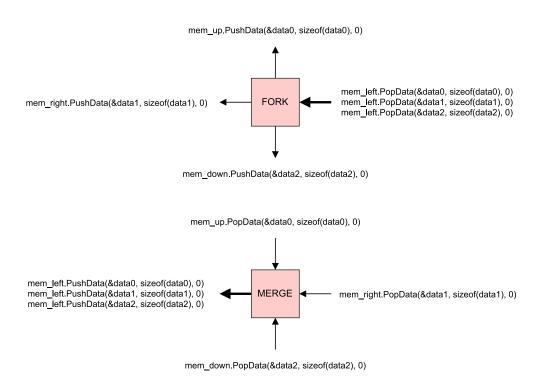
Figure 6: Fork and Merge operations with MemTools code.
