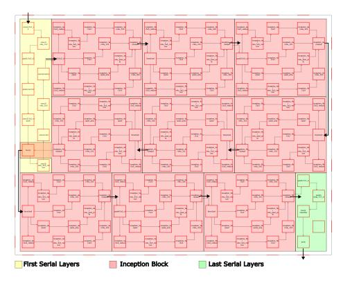
Figure 26: GoogLeNet CNN on GPC (version 2) structure.
