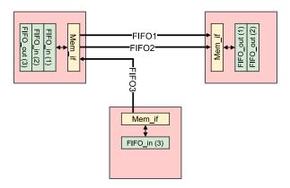
Figure 14: Example of communication between cores using MARI library, Channels View.
