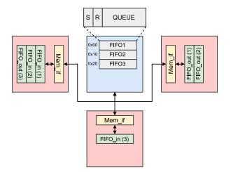
Figure 15: Example of communication between cores using MARI library, Memories View.
