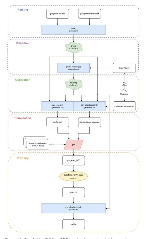
Figure 10: GoogLeNet CNN on GPC (version 1) complete implementation steps.
