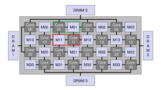
Figure 2: Representation of a 4 by 4 GPC model with "OFF-chip" DRAM memories [7].
