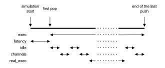
Figure 24: Module life span with delays contributions.
