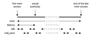
Figure 23: Channel communication life span with delays contributions.
