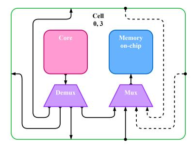
Figure 5: High-level Schematic of Corner Cell03 Inside Checkerboard without Adjacent Core on Top and Right, figure modified from [20]
