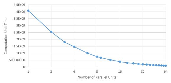
Figure 24: Mandelbrot on Checkerboard Model Computation Unit Time vs. Number of Parallel Units
