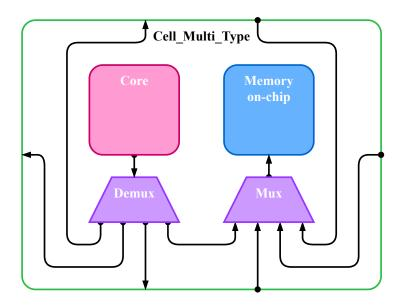
Figure 3: High-level Schematic of a Generic Multi-Type Cell Inside Checkerboard with Core & Core Demux on Left and Memory & Mem Mux on Right, figure modified from [20]
