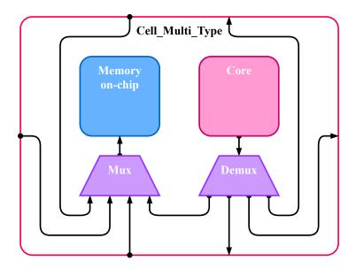
Figure 4: High-level Schematic of a Generic Multi-Type Cell Inside Checkerboard with Core & Core Demux on Right and Memory & Mem Mux on Left, figure modified from [20]
