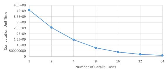
Figure 22: Mandelbrot Set Visualization 1.0 Model Computation Unit Time vs. Number of Parallel Units
