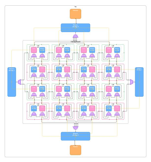
Figure 18: High-level Schematic of Mandelbrot on Checkerboard 4x4 Model, figure modified from [20]
