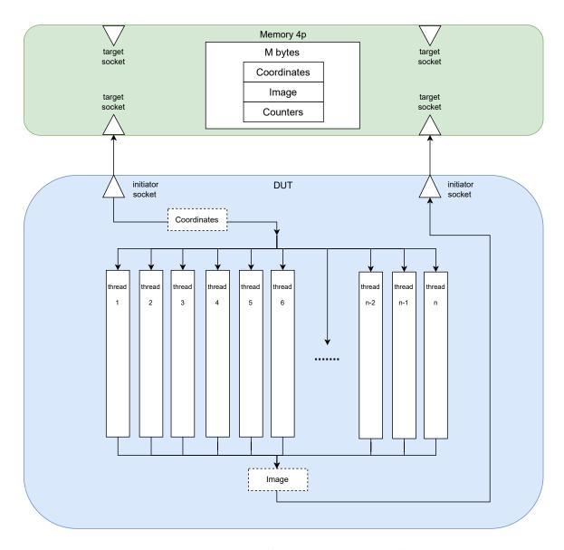
Figure 17: DUT schematic of 1.0 Mandelbrot Set Visualization
