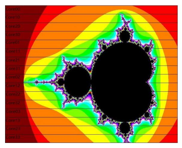
Figure 20: Mandelbrot Slices assigned to GPC Cores
