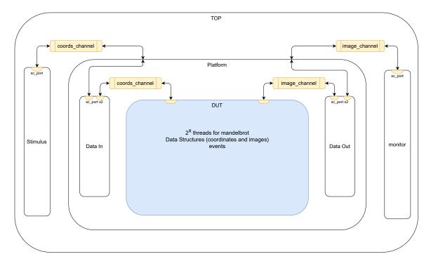
Figure 10: High Level Schematic of Base Model of Mandelbrot Set Visualization
