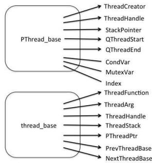
(a) Data Structures for kernel-level Threads and user-level Threads
