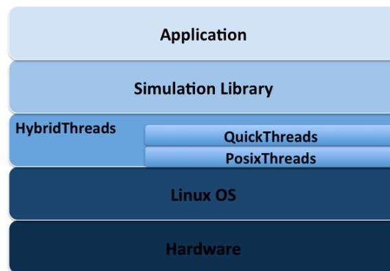
Figure 12: New Software Stack of SpecC Parallel Simulators
