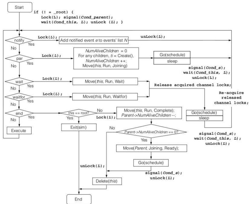
Figure 5: Lifecycle of a Thread in Parallel Discrete Event Simulation [6]
