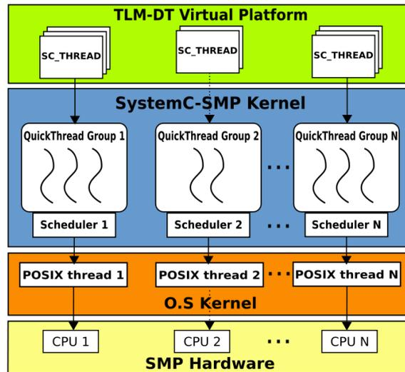
Figure 8: Software Architecture of the SystemC Distributed Simulator [17]
