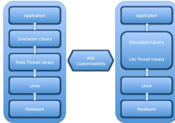
Figure 9: Software Stack of SpecC Parallel Simulator using LiteThreads [16]
