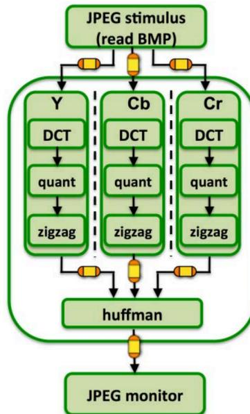
Figure 34: Block Diagram for JPEG Encoder [5]
