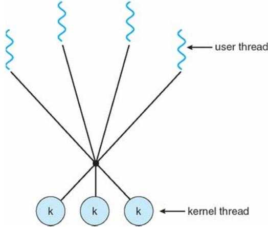
Figure 11: HybridThreads Threading Model [19]
