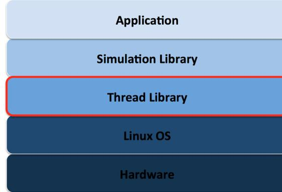
Figure 6: Software Stack of SpecC Simulators
