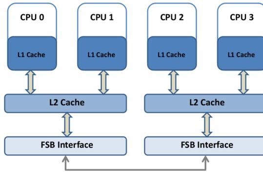
Figure 25: Intel Core 2 Quad architecture, Q9650 (mu) [14]
