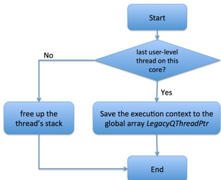
Figure 22: Control Flow of ThreadDelete
