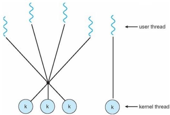
Figure 51: Two Level Threading Model [19]
