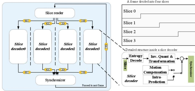
Figure 39: Block Diagram of H.264 AVC Decoder [9]
