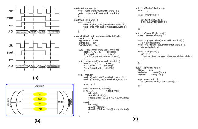
Figure 5: Synchronous bus channel
