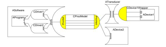
Figure 10: Model of a microprocessor system with IO devices.
