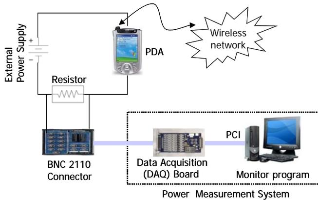
Figure 6. Experimental setup for power measurement
