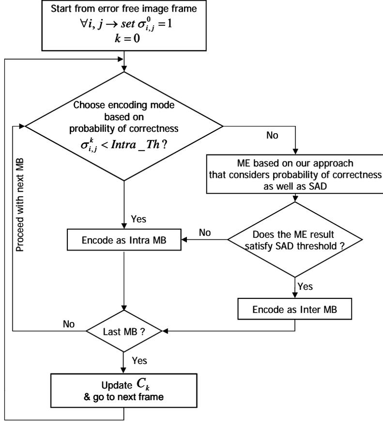
**Figure 2. PBPAIR error resilient coding**
