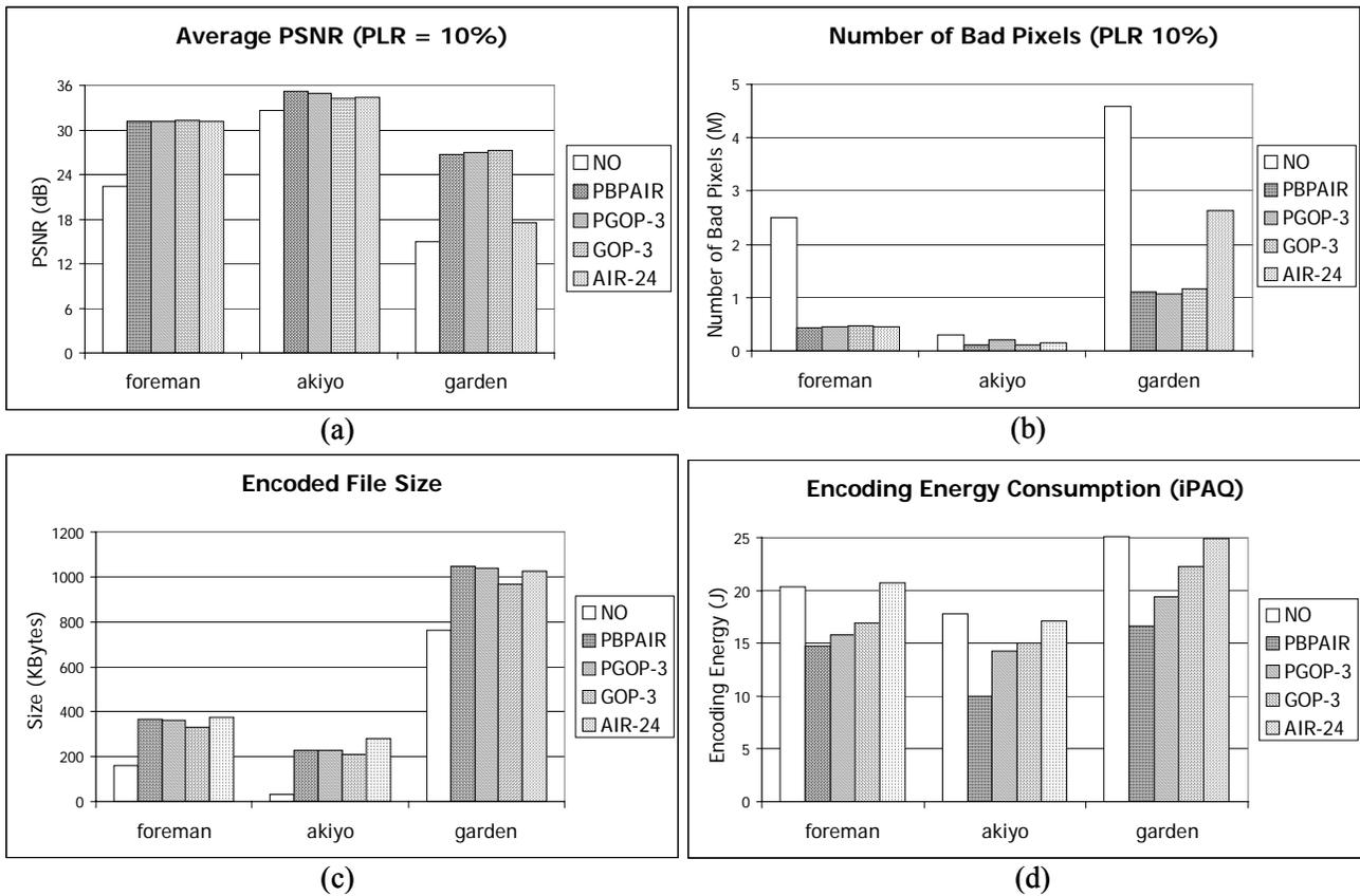
**Figure 7. Comparison between PBPAIR and existing error resilient techniques such as PGOP, GOP, and AIR, where PLR is assumed to be 10%: (a) the average PSNR (b) the number of bad pixels as an image quality measure (c) the encoded file size (d) the encoding energy consumption using iPAQ as a performance measure (image source: FOREMAN.QCIF, AKIYO.QCIF, and GARDEN.QCIF, 300 frames)**
