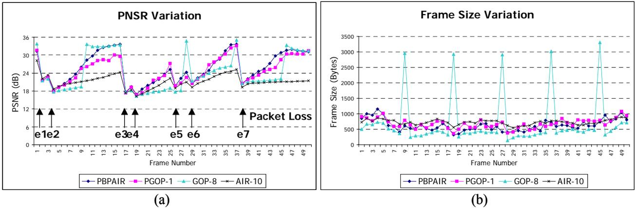
**Figure 8. Comparison between PBPAIR and existing error resilient techniques such as PGOP, GOP, and AIR, where PLR is assumed to be 10%: (a) PSNR variation (b) frame size variation (image source: FOREMAN.QCIF, 300 frames)**
