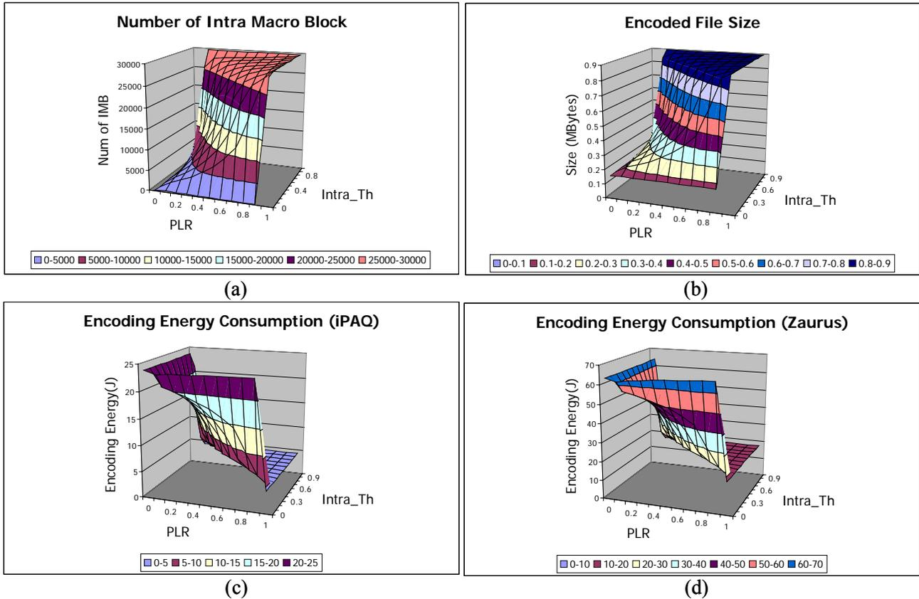
**Figure 9. Trade-offs on varying PLR and *Intra\_Th*: (a) the number of intra MBs (b) encoded file size (c) encoding energy consumption in the case of iPAQ (d) encoding energy consumption in the case of Zaurus (image source: FOREMAN.QCIF, 300 frames)**
