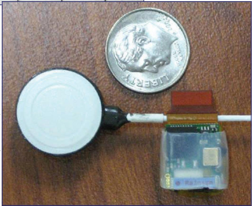
nication links for wearable medical sensors. The industry sponsor is QUASAR, Inc., in San Diego, CA (<http://www.quasarusa.com/>). QUASAR is the maker of new types of ECG, EEG, and many other novel medical sensors.
