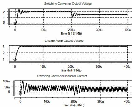
Figure 4. simulated waveforms during DVS transient
