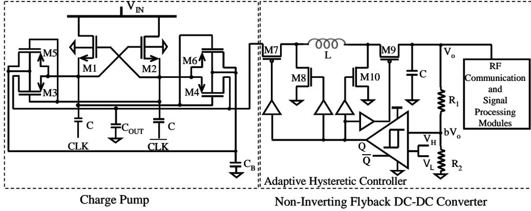
Figure 2. Schematic of a simplified power regulation system
