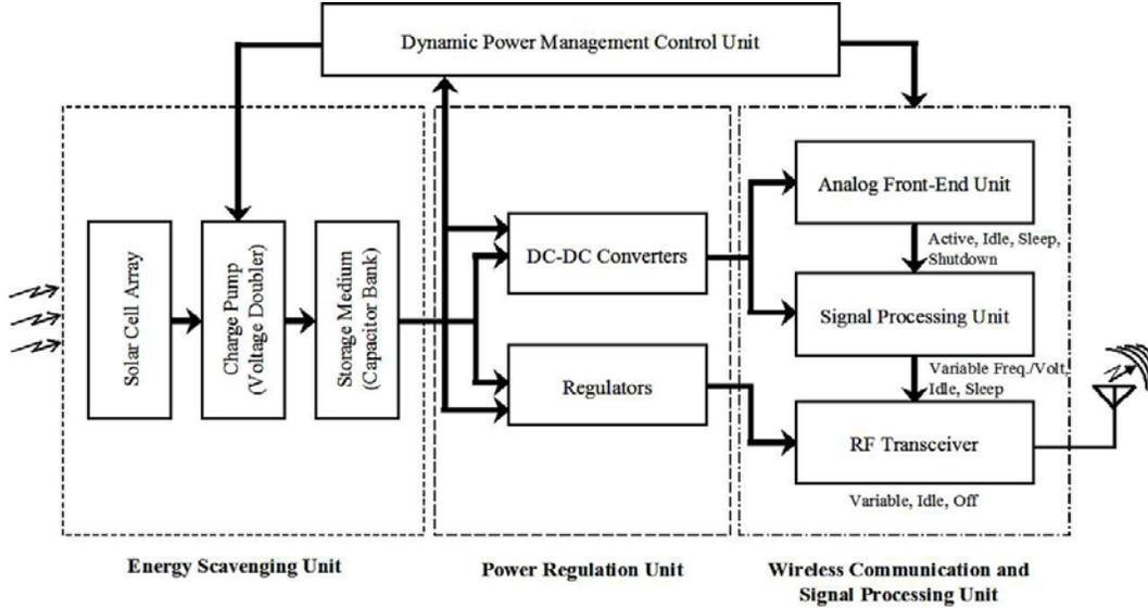
Figure 1 Block diagram of the proposed wireless sensing node
