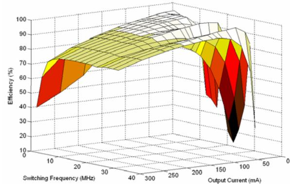
Figure 6. Efficiency versus switching frequency of charge pump
