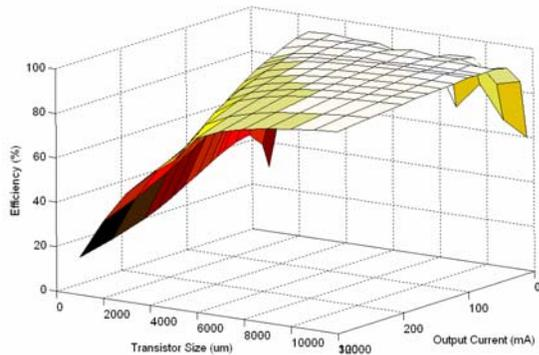
Figure 5. Efficiency vs transistor size of SMPC converter
