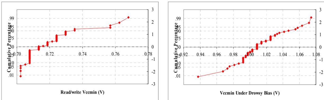
**Figure 5:** The measured Vccmin with active read and write operation and standby condition with drowsy back bias. Note the Vccmin is higher with drowsy bias. As the Vccmin tracks the high rail supply, the drowsy Vccmin is elevated as the Vss of the cell is raised with back bias.
