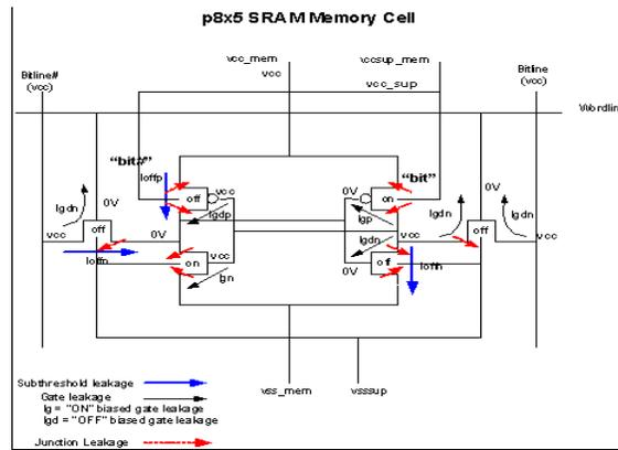
Figure 3: Cell leakage components and leakage paths during drowsy back-bias.
