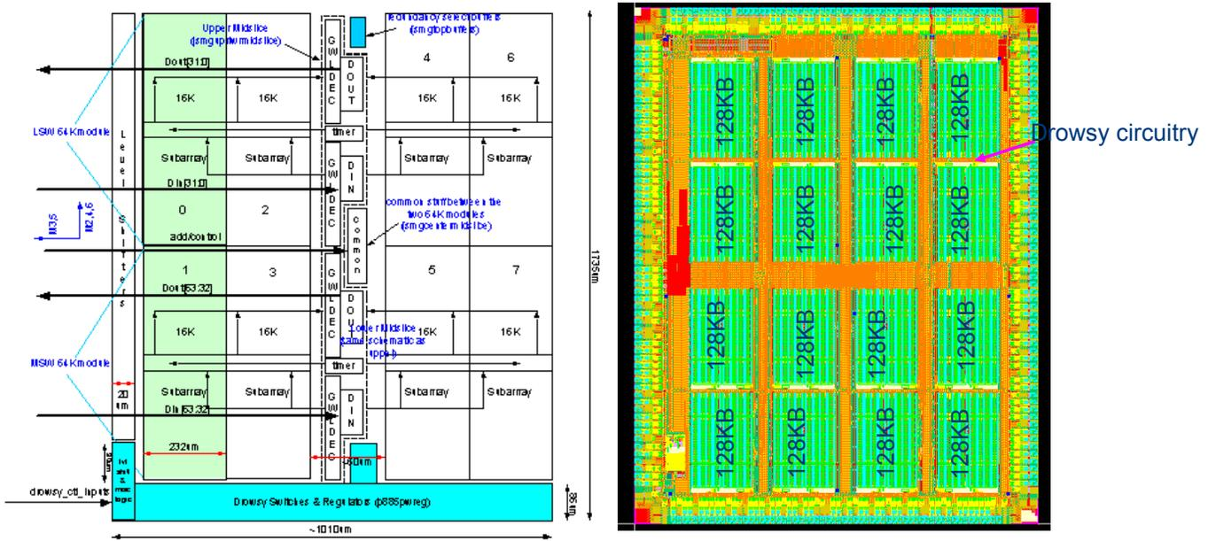
Figure 1: Block diagram and layout of the of the 2MByte SRAM testchip.
