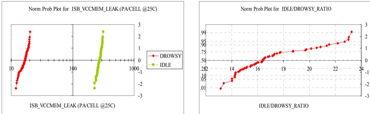
**Figure 4:** Measured cell leakage during idle and drowsy back bias. The optimized PMOS and NMOS back bias for good retention led to a cell current of only 20pA at 1.3V, 25C. The Measured median Idle/Drowsy leakage ratio is 16.
