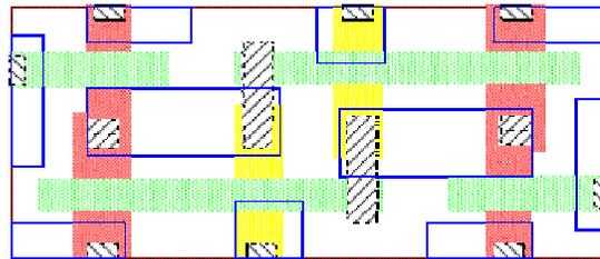
Figure 2: Layout of the wide bit cell.
