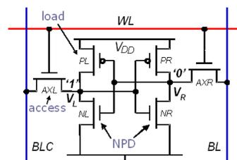
Figure 1. Schematic of a conventional 6-T SRAM cell.
