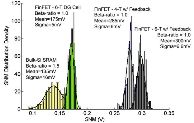
**Figure 12. Impact of process variations on SNM. Cell designs with dynamic feedback have improved noise margin than the standard 6-T DG-SRAM. Dopant induced fluctuations cause larger SNM spreads in the bulk devices.**
