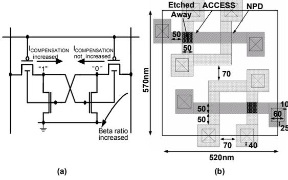
**Figure 9. Circuit schematic (a) and layout (b) for a 4-T SRAM cell with back-gate connections to provide dynamic feedback. Note the use of BG-FinFET PMOS access devices, indicated in the layout by a dark layer over their gate electrodes.**
