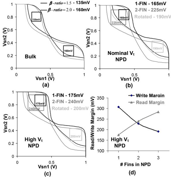
Figure 6. 6-T SRAM read butterfly plots (a) bulk-Si MOSFET SRAM cell with  $\beta$ -ratio = 1.5 (black), 2.0 (gray) and (b-c) FinFET-based SRAM cell with 1-fin (black), 2-fins (dark gray), and rotation (light gray). (d) Impact of adding fins to the NPD on the read- and write-margins.
