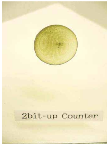
Figure 9. Sample context of a two-bit up-counter and the photograph of a holographic memory recorded with the context.
