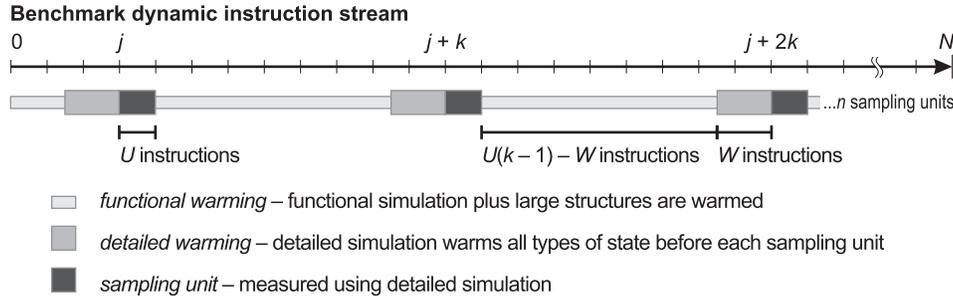
**Figure 2. Systematic sampling as performed in SMARTS.** Two modes of simulation are used: functional simulation, and detailed simulation. The need to determine warmup requirements for large structures, such as caches, is eliminated by performing continuous functional warming.
