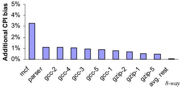
**Figure 3. Restricted live-state bias.** If only correct-path state is stored, wrong-path instructions are not accurately simulated.
