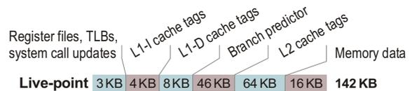
**Figure 4. Breakdown of a typical live-point (uncompressed).** For comparison, a conventional checkpoint is 105 MB on average.
