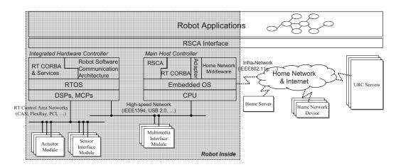
Figure 1. Structure of hardware and software of URC robot.
