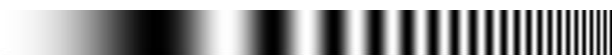
Fig. 1: The basic MTF test pattern, a sine wave of increasing spatial frequency.
