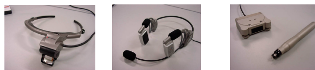
(a) See-through HMD (b) bone conduction speaker (c) 2D-pen sensor
