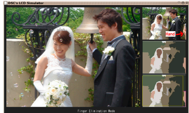
Fig. 1. Overview of the autoframing recommendation system: Once the system has detected undesirable objects in pictures (here, a hand indicated by a bold arrow), it automatically crops the picture while preserving the aspect ratio.
