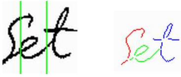
Fig. 2. Character segmentation for handwritten word “set”. Left image: Segmentation with vertical cut. Right image: Stroke-based segmentation, with different colors showing characters segmented at stroke boundaries.
