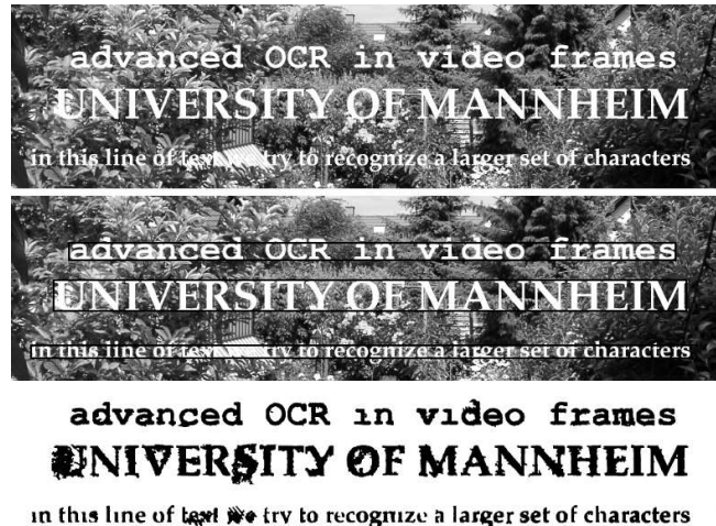
Fig. 6. Original image (top), automatically detected text regions (center) and segmented text (bottom)
