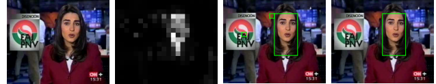
Fig. 3. Example of the proposed approach to skin color segmentation for face detection in the compressed domain. From left to right: original images, likelihood of each block w.r.t. the Gaussian skin color distribution in the Cb-Cr space (rescaled for proper visualization), results of skin color segmentation (step 1 of our attentional cascade), results after filtering bounding box size and aspect ratio (step 2 of the cascade).
