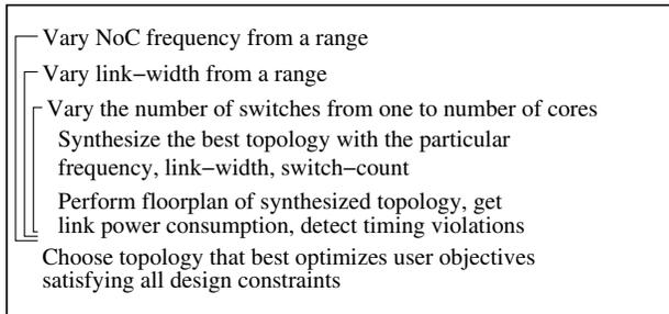
Figure 2: NoC architecture synthesis (phase 2 of design flow)
