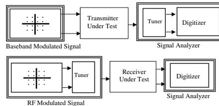
Figure 3: EVM measurement setup
