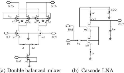
**Figure 5: Transistor level mixer and LNA circuit**
