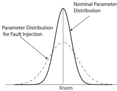
**Figure 4: The distribution of circuit level and block level parameters used in Monte Carlo simulations**
