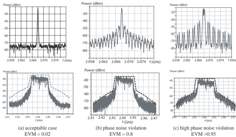
Figure 6: Bench measurement results for a good chip and two faulty chips
