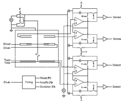
Figure 5. Schematic of the on-chip electronics of the integrated gyroscope of Fig. 4 [15].
