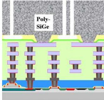
Figure 3. Schematic cross-section of the integrated gyroscope.
