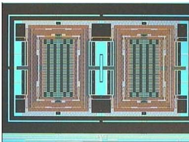
Figure 4. Photograph of the poly-SiGe gyroscope processed on top of a standard  $0.35\text{ }\mu\text{m}$  CMOS process with 5 metal levels [15].
