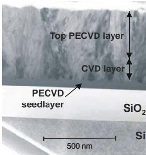
Figure 2. Cross-section of the PECVD/CVD poly-SiGe multilayer [9].
