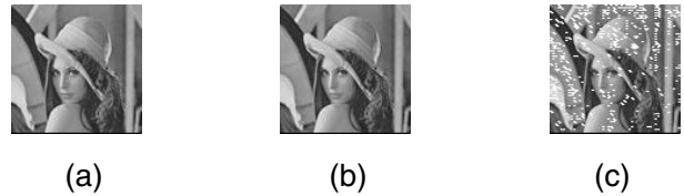
Figure 8: (a) Conventional correct operation (baseline) (b) Non uniformly voltage overscaled case, with saving of 21.7% in energy when compared to the baseline (c) Conventional uniformly voltage overscaled case for the same energy as (b)
