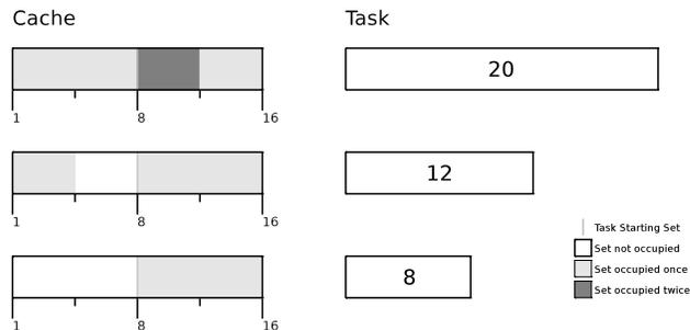
**Figure 2:** Shows a 16kb cache and three different tasks with different sizes. Each task starts at the same cache set.
