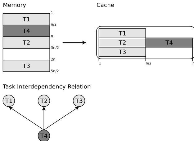
**Figure 3: Optimal placement of four tasks for a direct-mapped cache comprising  $n$  sets with respect to the given task interdependency relation. Each of the tasks occupies half of the cache.**
