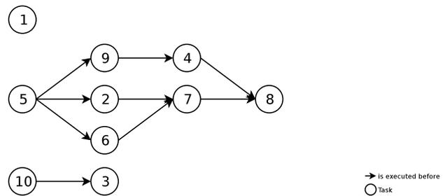
Figure 5: Shows the structure of the task sets A, B and C. Incoming edges denote which tasks have to be completed before a task may begin.
