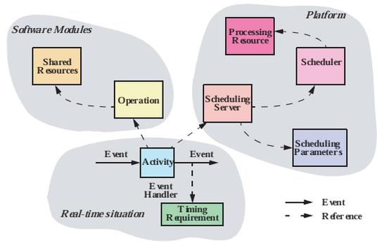
Figure 5: Elements of the MAST model
