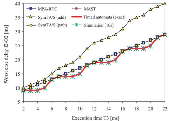
Figure 12: Analysis results for the worst case delay I2-O2 in benchmark 2
