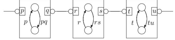
Figure 11: Synchronous modulo-8 counter.
