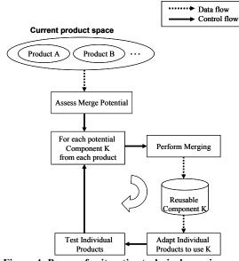
Figure 4: Process for iterative technical merging.
