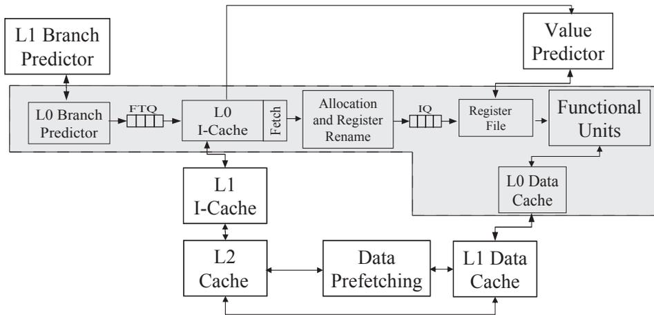
Figure 1: The single core architecture explored in this study.
