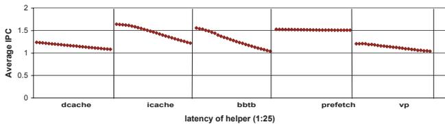
Figure 4: Impact of Latency on Our Helper Engines
