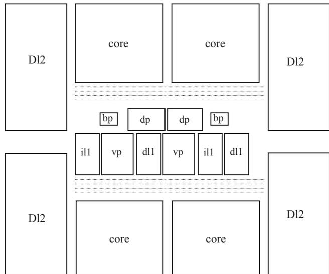
Figure 5: Our CMP floorplan, with cores and L2 cache banks distributed around 2 sets of helpers.
