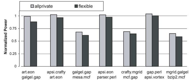
Figure 11: Power dissipated in flexible and allprivate configurations normalized to baseline configuration with shared helpers.
