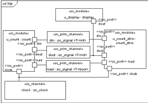
Figure 4: Example of a Composite Structure
