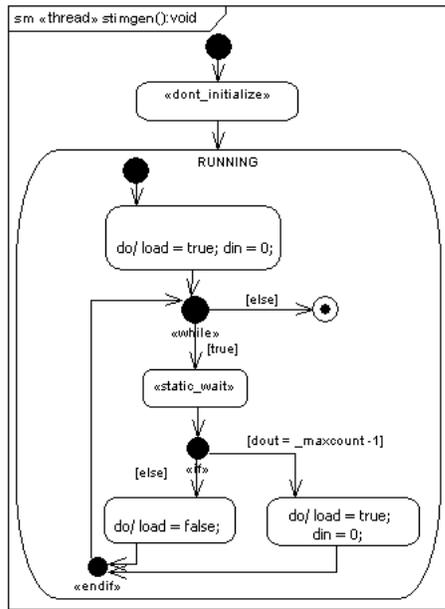
Figure 7: A thread process state machine
