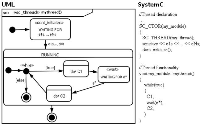
Figure 6: A Thread Process pattern
