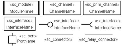
Figure 2: Structure Stereotypes Notation
