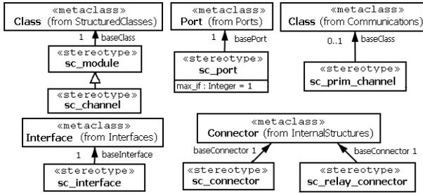
Figure 1: Structure Stereotypes Definition
