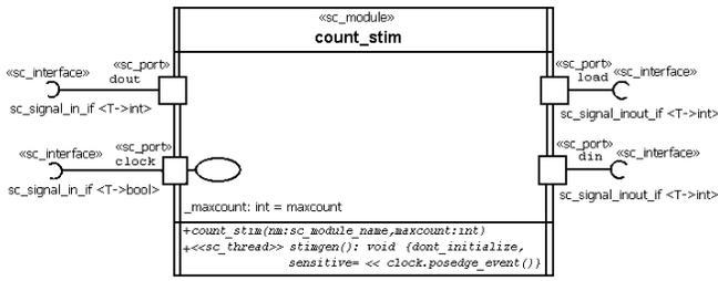
Figure 3: Example of a module, its attributes, functions, processes and ports
