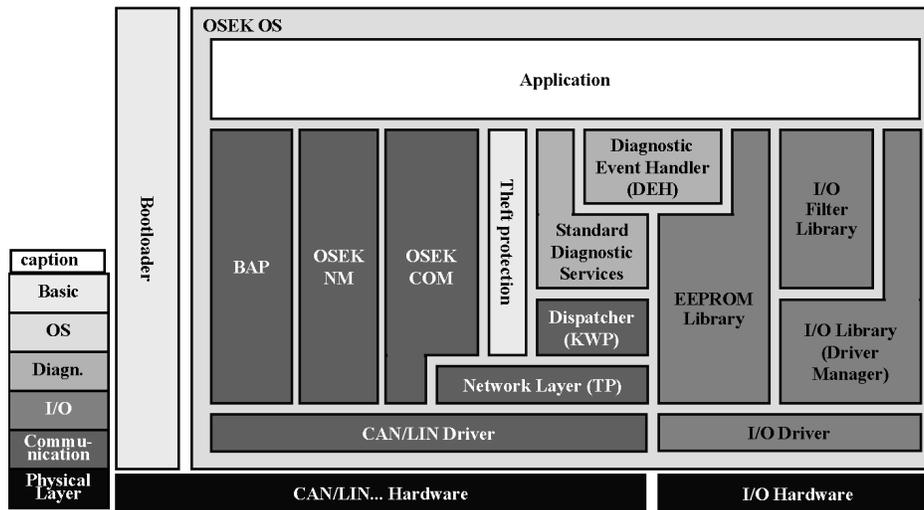
Figure 6: Example of a Standard Software Core (SSC)
