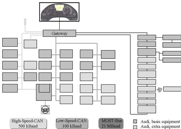
Figure 2: Electronic System of the AUDI A8
