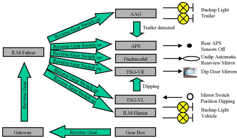
Figure 11: Example Reverse Gear
