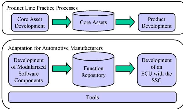
**Figure 3: Modules of the Framework for the Reuse of Software Components for Automotive Manufacturers**
