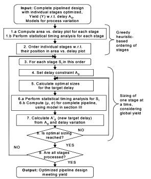
Figure 9: Algorithm for the global optimization of pipeline for ensuring yield with minimum area overhead
