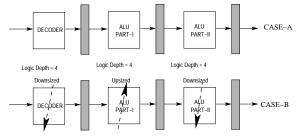
Figure 6: A 3-stage pipeline with different stage delays
