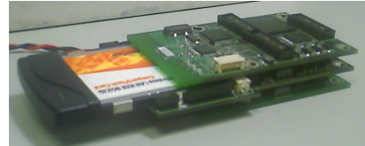
Figure 1. An mPlatform node with the 802.11 and 802.15.4 radios.
